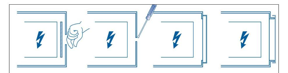
The IP code for this example without the barrier is IP1X, but with the internal barrier fitted as shown it can become IP1XC or even IP1XD.
