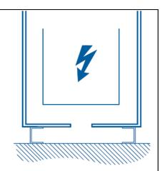
The IP rating can be affected by the installation position; here the mounting surface acts as an external barrier and limits accessibility.
