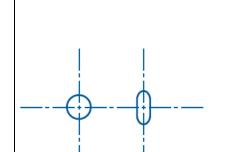
The minimum recommended aperture sizes to allow for drainage and overcome the surface tension of water are 5.0mm diameter, or a 3.0mm width slot of 20.0mm<sup>2</sup> area.
