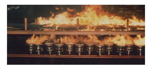
Typical Fire Testing standards for electrical components was directly from both the Piper Alpha explosion in the North Sea as well as the Chunnel fire in the UK. Health and safety regulations require certain products for use in critical areas must meet specific fire testing requirements. IEC has also the same requirements for critical circuits such as IEC331 and IEC332 rating for cables. The specific testing requirements are as followed:
